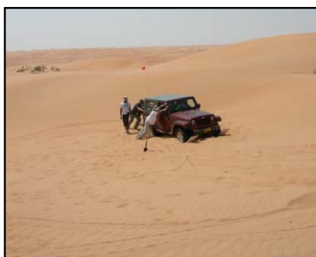
Check out the tracks, this jeep has gone in a circle trying to maintain speed and momentum but has lost the fight. An ideal case for sand ladders as bringing another car in to tow could easily result in two stuck vehicles.
