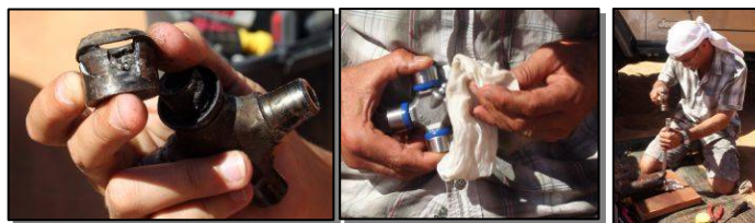
This set of photos shows our technical officer Simon Hatfield replacing a damaged CV joint 'over lunch' on a recent trip. This one had failed due to lack of adequate lubrication.
