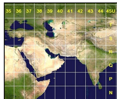
The UTM grid for the M East region showing Oman in the 40Q 'zone'. Beyond this each zone is divided into northing and easting coordinates based on 'metres' from the bottom and left boundary
